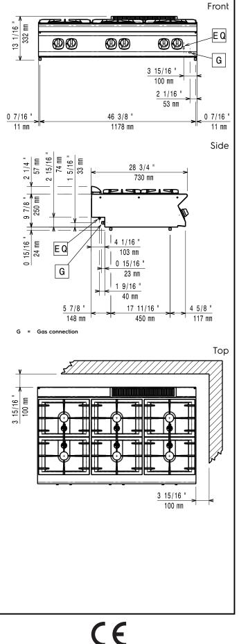
Modular Cooking Range Line 700XP 6-Burner Gas Boiling Top
